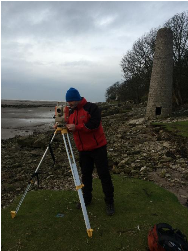
Plate 31. Furness Mapping Services undertaking a topographic survey to record extent of saltmarsh/erosion at Site 2, December 2015
