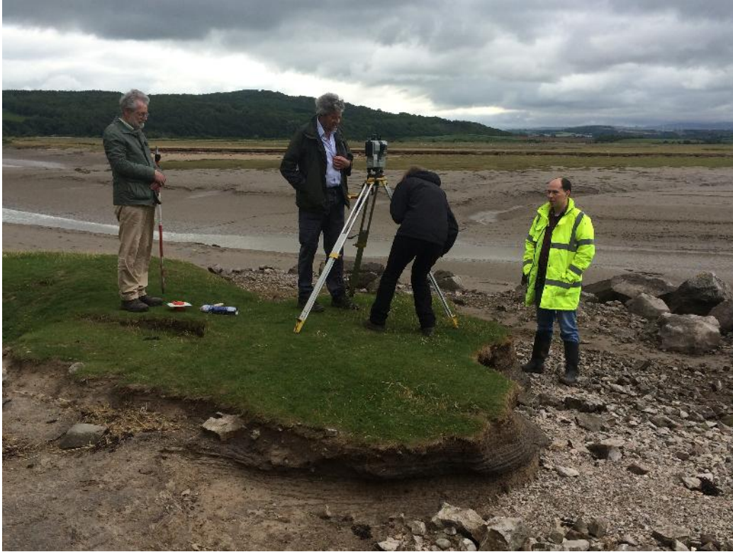
Plate 27. Jamie Quartermaine of Oxford Archaeology North and Andy Sherman of CITiZAN setting up survey stations and demonstrating the use of a Total Station Theodolite, looking south-west
